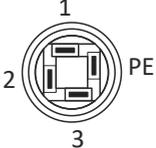
**Control connection X1 with M12 connector, A-coded, pins**
