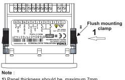
Panel thickness should be maximum 7mm.
